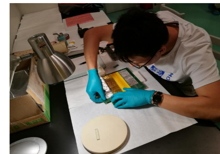
Strip wrapping and assembly on EBU was done by hand (Shanghai Institute of Ceramic)
