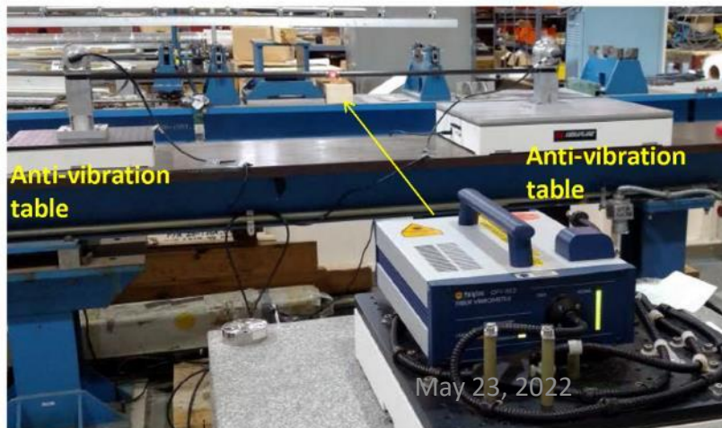
Vibration measurement system for SuperKEKB final focus magnet (KEK)
