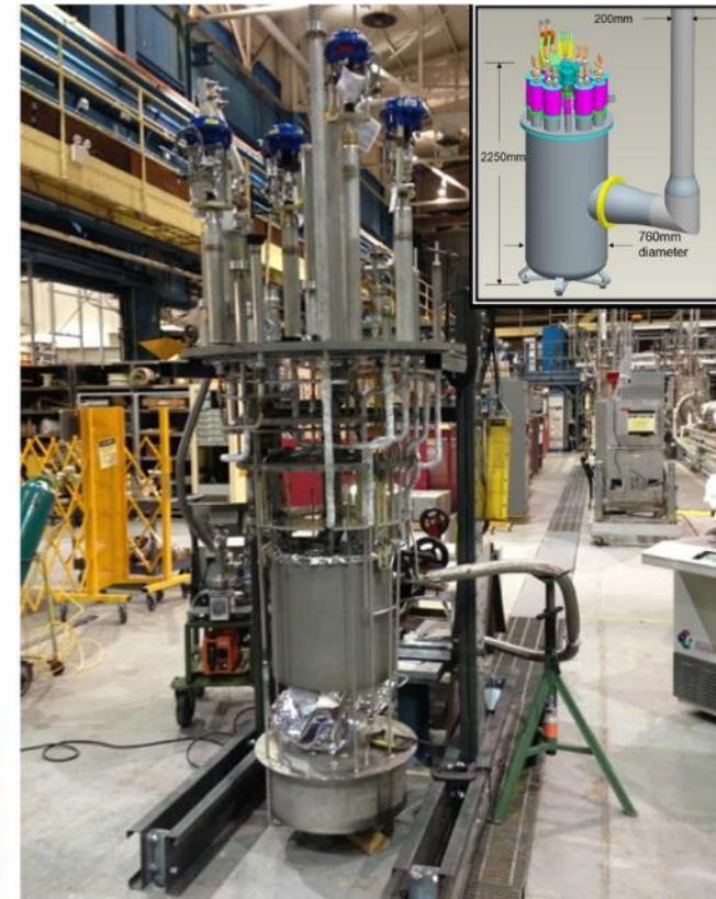
Prototype of ILC service cryostat ( 2K cooling system ; BNL )
