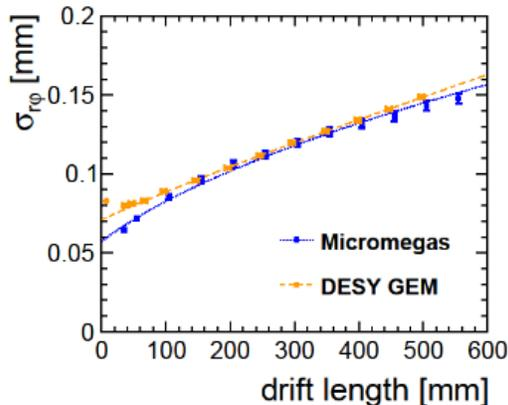
Figure 1: Comparison of transverse spatial resolution in dependence on drift distance for the pad-based technologies at  $B = 1$  T [8].
