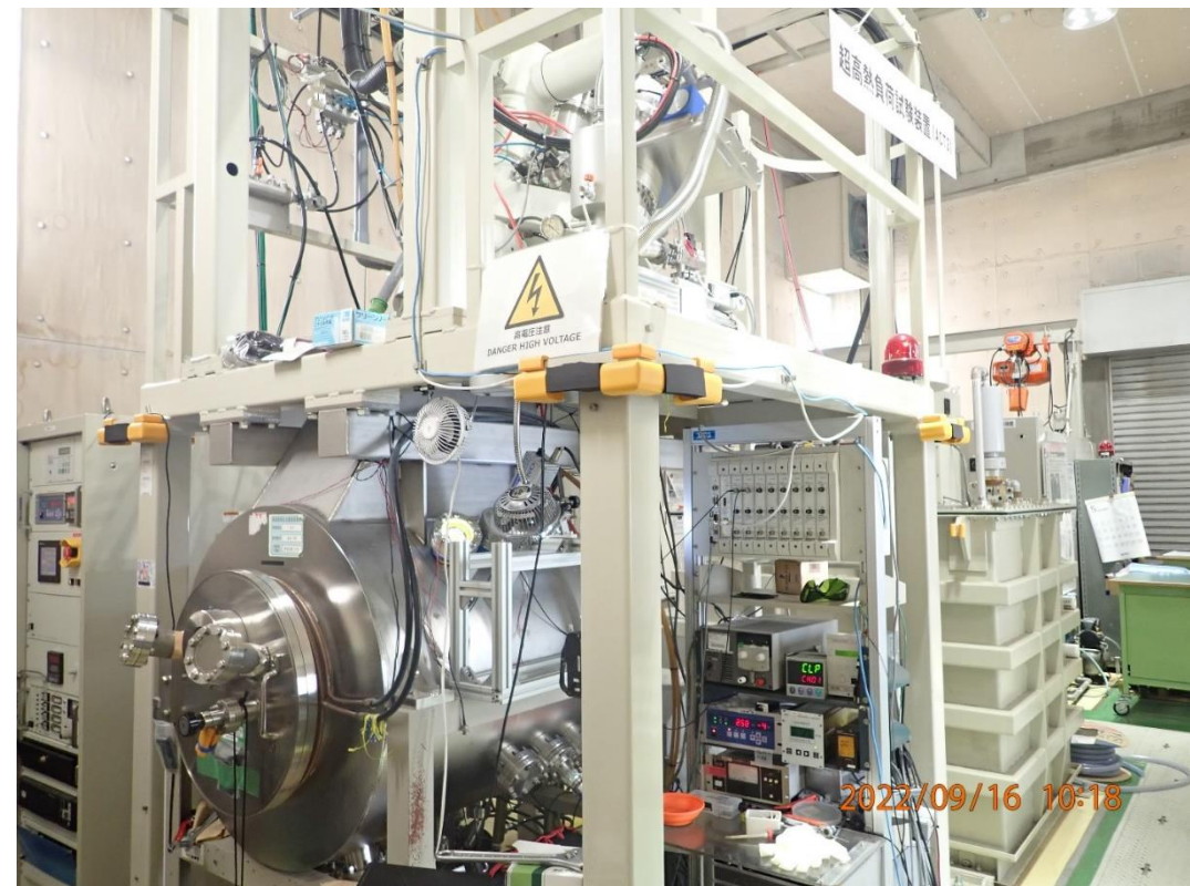
40 kV, 300 kW electron beam heating machine @ NIFS
