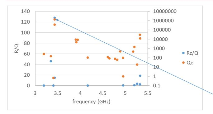
Waveguide damper does damp the pi and 0 modes well but doesn't damp the pi/2 modes but these will be damped strongly by a coax damper in the beampipes. Considering a waveguide section with a coax coupled to it to minimize size and heat leak. Coax can be positioned to prevent coupling to the crabbing mode.
