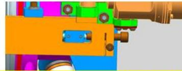
Function of this screw to unload tuner to replace piezo/motor
