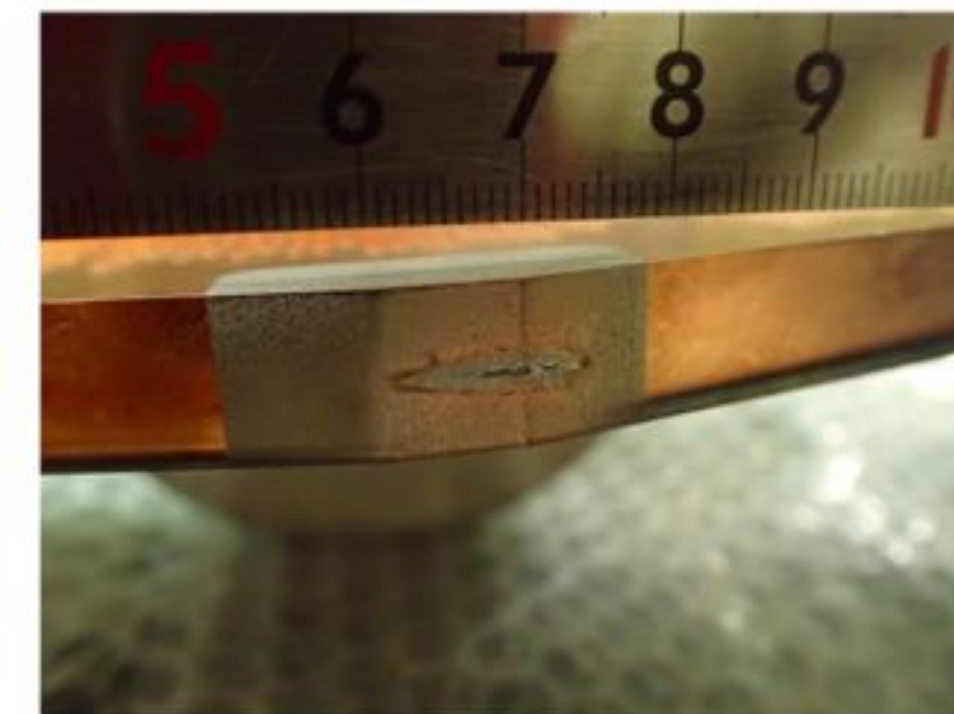
Damage to coated collimator jaw due to accidental beam loss in SuperKEKB
