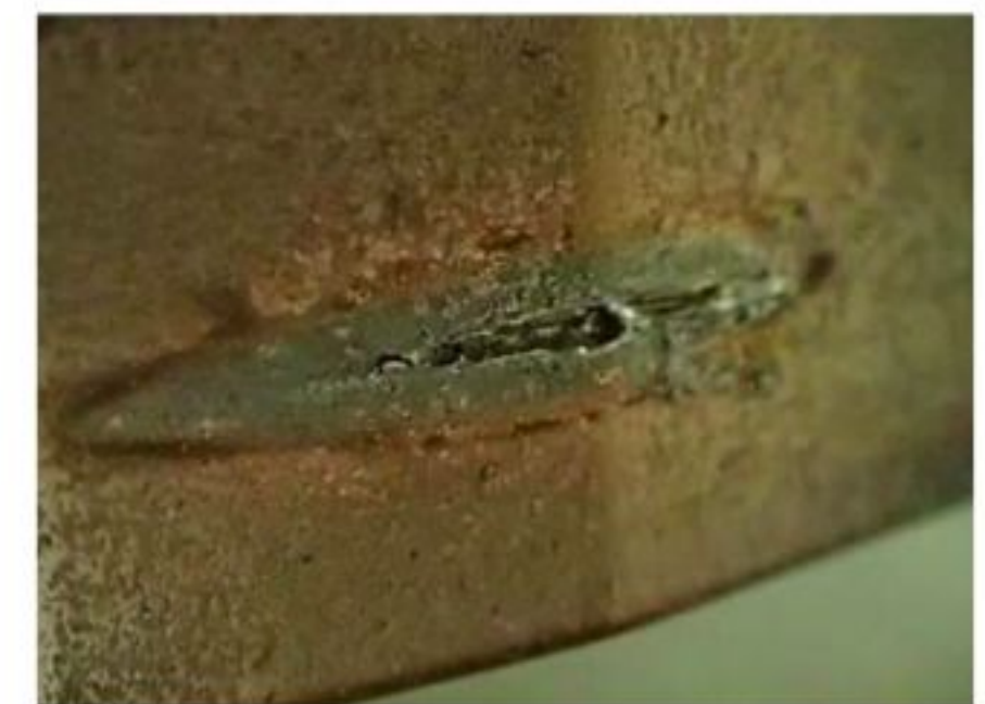
Damage to coated collimator jaw due to accidental beam loss in SuperKEKB
