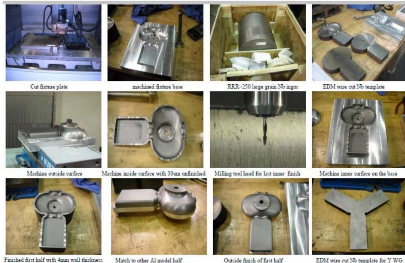
2.8 GHz SPX Cavity Fabrication at JLAB
