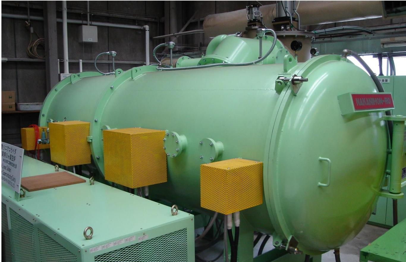
**Annealing / degassing furnace at KEK : Two 9-cell cavity can be processed at once. Designed to consider about the supper-structure (Super-structure is consisting of two connected 9-cell cavities with one input-coupler).**
